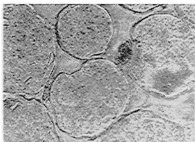
Photo. 3. Microphotograph of the cross-section of the fiber containing sample-G after acetone-extraction.
